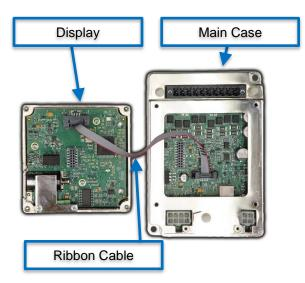
Figure B: Trip Unit and Display (separated)
