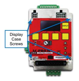
Figure A: Display Case Screw locations
